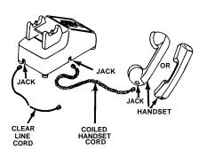
Figure 2. Desk Telephone Installation
